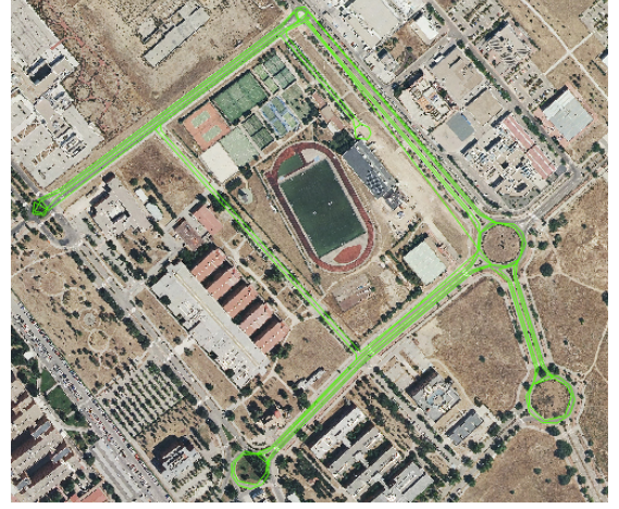
Fig. 9. Resulting mission plan (green) after applying NN algorithm.
