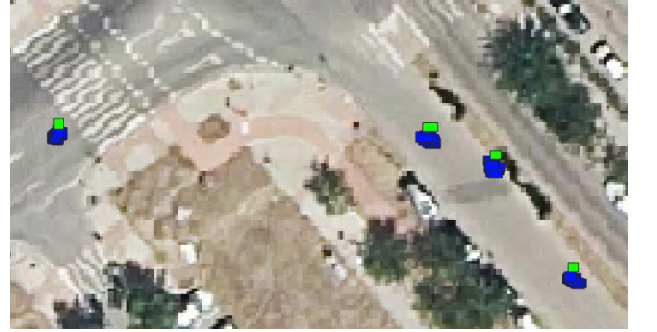
Fig. 14. Fourth system output example (green is ground truth and blue are predicted bounding boxes).
